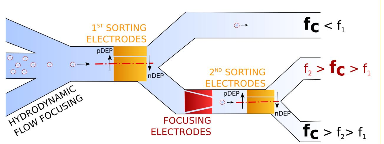
Cells tracing the middle path have the first crossover frequency in the designated frequency window (between the electric field frequency at the first sorting step and the second sorting step). The width of the frequency window is only limited by the sorting sensitivity. Different flow rates yield different sorting sensitivities. The active domain of the electric field gradient determines the absolute lower limit on the frequency window.
