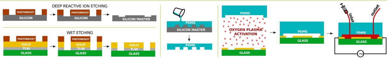
Another fabrication process is considered to avoid the PDMS misalignment. The channel walls may be formed on top of the glass substrate by layer of the SU-8 photoresist. Then, the channel can be sealed by flat piece of PDMS. Before sealing, SU-8 and PDMS surfaces must be exposed to oxygen plasma to ensure proper sealing as in the case of previous fabrication process.
