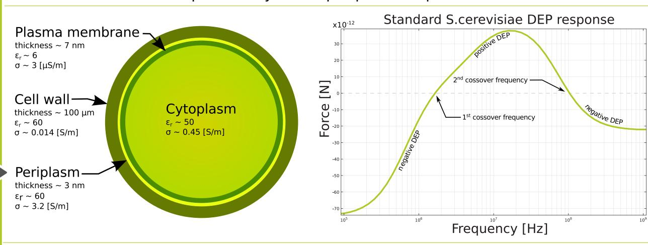
The standard dielectrophoretic response of a Saccharomyces cerevisiae cell shows the magnitude and the direction of the induced force is controllable through electric field frequency modulation. Hypothesized dielectric reporter proteins are polypeptide molecules that significantly change the dielectrophoretic response. This change can be harnessed for cell sorting according to reporter protein concentrations.
